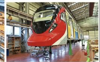
The SSP Line has a total of 49 trains. Instead of stainless steel, the car bodies are made of aluminium.
